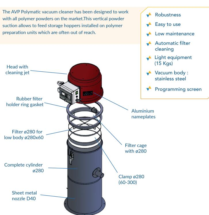
Thanks to this suction system, operators no longer need to lift heavy bags into high, inaccessible hoppers. This system can be adapted to all of our units, as well as others...
